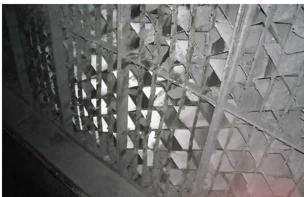
Figure 1. Coke formation in the coker wash bed after three years of operation.
