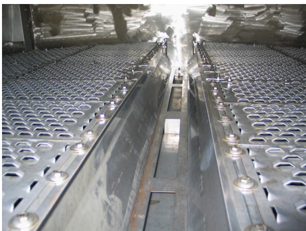
Figure 2. Sulzer VG AF TM anti-fouling trays with SVG TM , push valves and enhanced outlet weirs.
